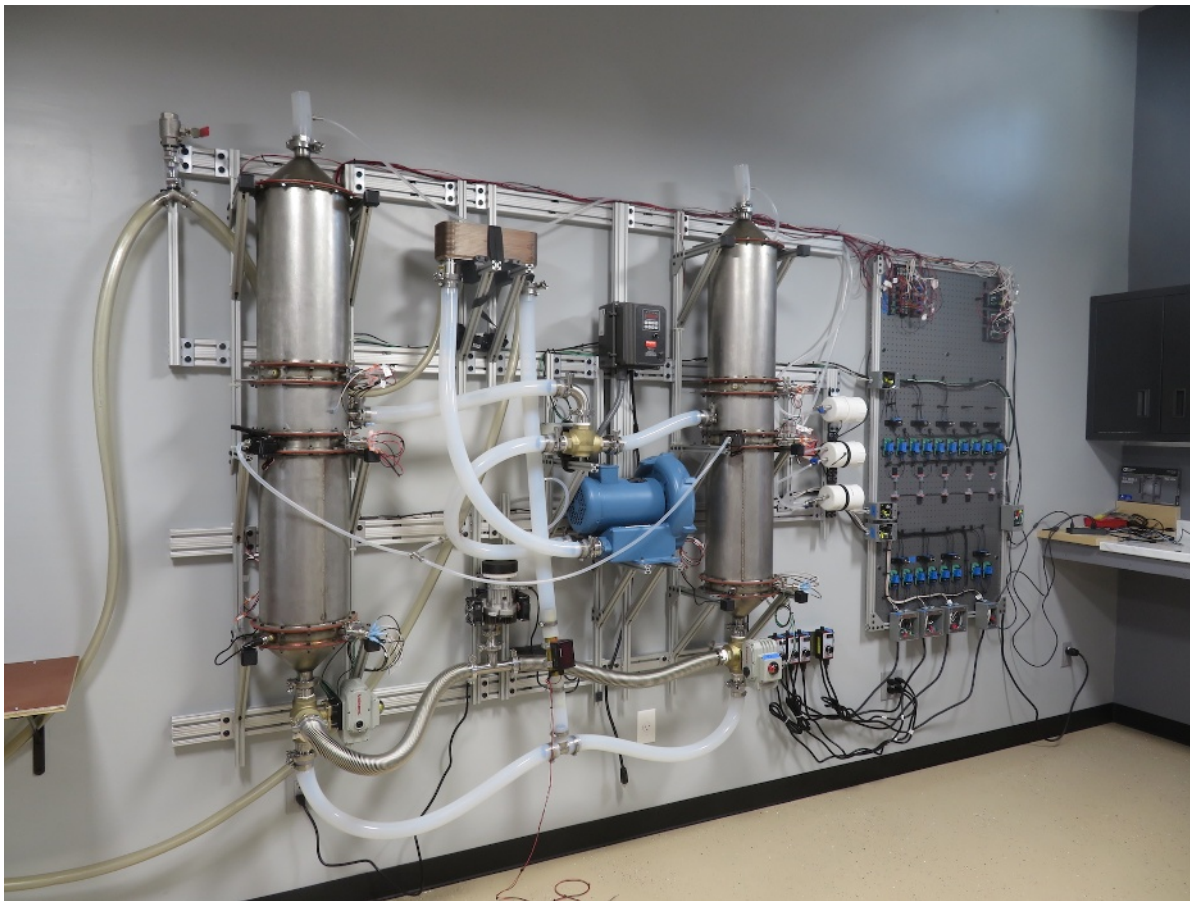
Figure 9. SAM Carbon Dioxide Removal Assembly.
